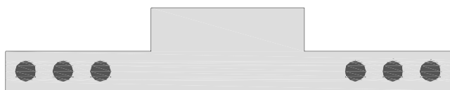
Reverse T-Bar with (6) 4 in. Round Light Holes
