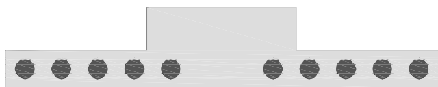
Reverse T-Bar with (10) 4 in. Round Light Holes
